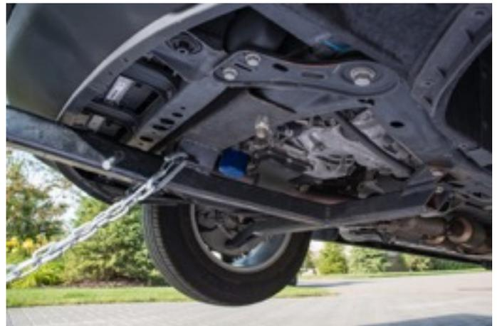
Determine the elevation under the towed vehicles frame and make sure you will have an unobstructed elevation to the front of the towed vehicle and make sure the ground clearance is adequate for safe operation of the vehicle. Make the spacers if needed, drill hole and female threads to match the supplied bolts in all of the spacer blocks. Once you are satisfied with your measurements (double check) weld the junction of the T-Joint.
